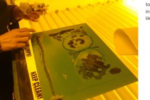
After the exposure you have to take off parts that might interfere with the developer, like tape.
