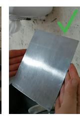
You can also use potato. In this case you do not wet the plate first, but you immediately rub potato onto plate and then rinse with water.
