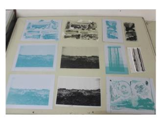
In this tests we used 37 seconds of exposure, except the line drawing that was verified from 10 to 70 seconds.
