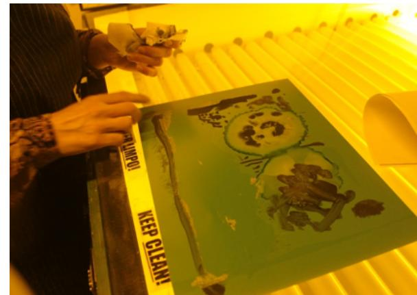
After the exposure you have to take off parts that might interfere with the developer, like tape.
