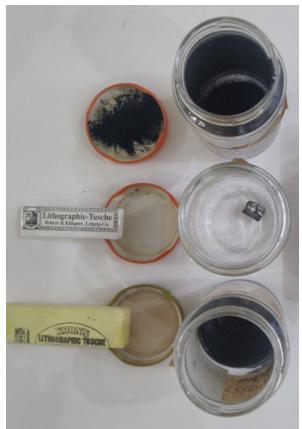
Testing tonal range by using toner powder and lithographic tusche, mixed with alcohol and with distilled water.
